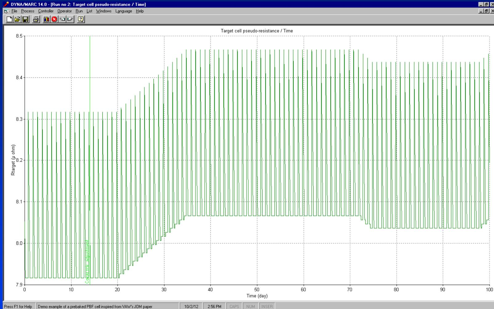
Evolution of the cell target resistance (there is a 0.4 micro-ohm change of target resistance each day during the anode change event).
