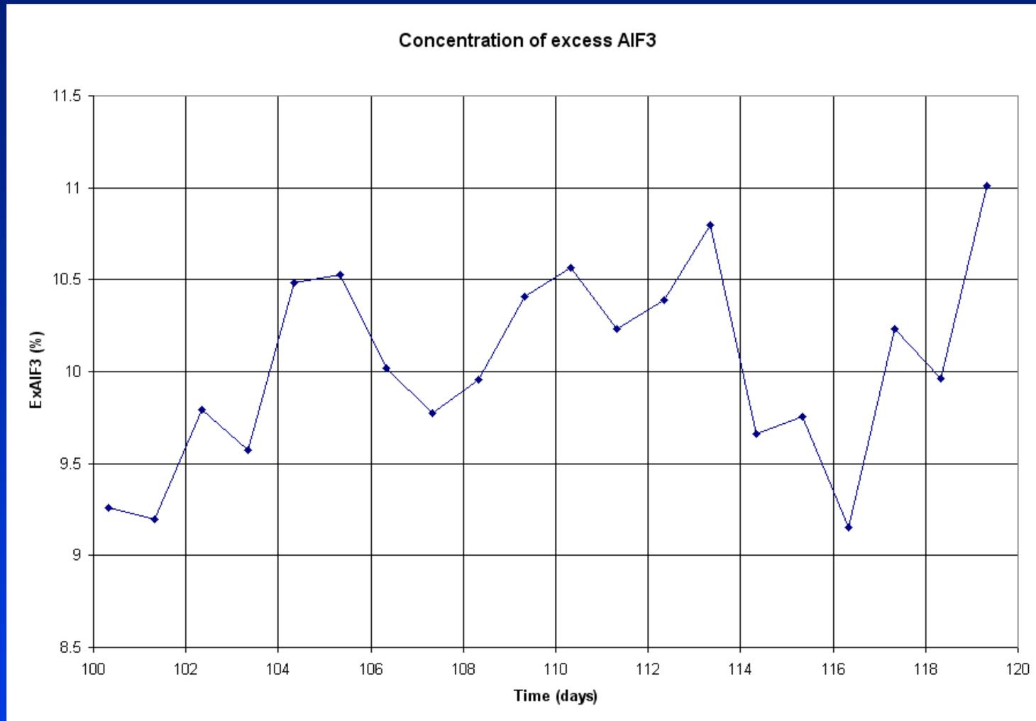
Figure above shows the results of bath sampling performed on the 20 days period when a 0.5% standard deviation white noise is added to the noise free results
