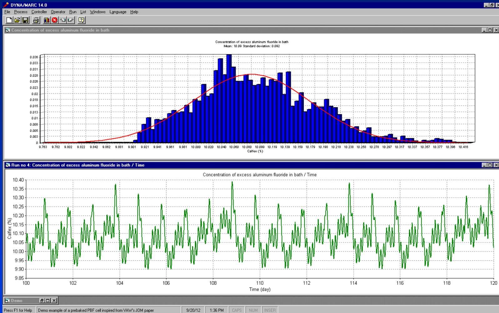
Figure above shows the variation of the  $AlF_3$  for a period of 20 days again without control and any mass imbalance.
