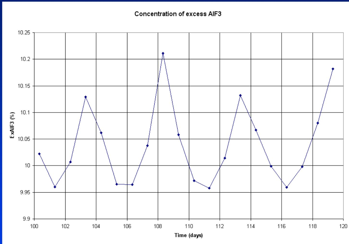
Corresponding 20 days of excess AlF<sub>3</sub> concentration sampling results assuming no bath sampling noise.
