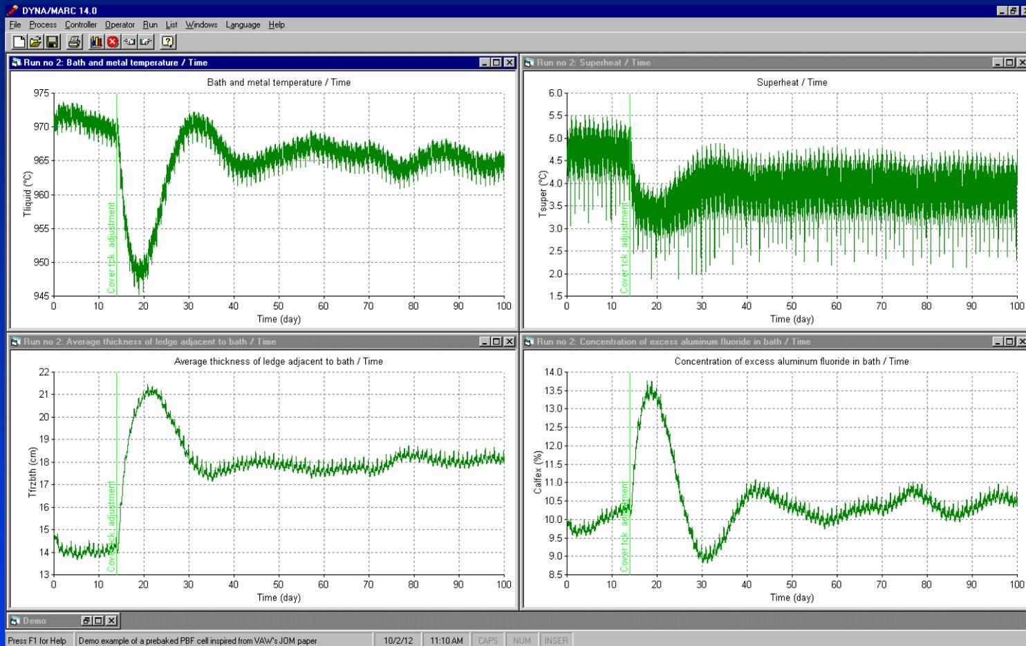
Simulation of the process with a significant perturbation; feedback control, 10% target concentration: STARprobe™ measurements once per day, 0.5 kg/hr% proportional band and daily 0.1 micro-ohm target resistance correction due to superheat offset from target.
